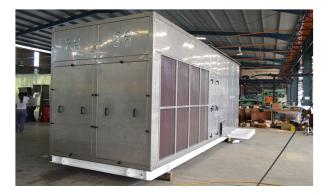
SPECIFICATION Full SSTL Casing Cu-cu heresite coil Tandem Scroll compressor PAGAS blade propeller fan Backwark incline explosion blower 100RT Package Unit
