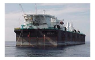
Floating, Storage , and offloading (FSO), Puteri Dulang. FSO Puteri Dulang is 128697 MT DWT, Single Hull with Cargo Capacity of 138931 M3. Equipped with the necessary accommodation and life support facilities for 60 persons.
